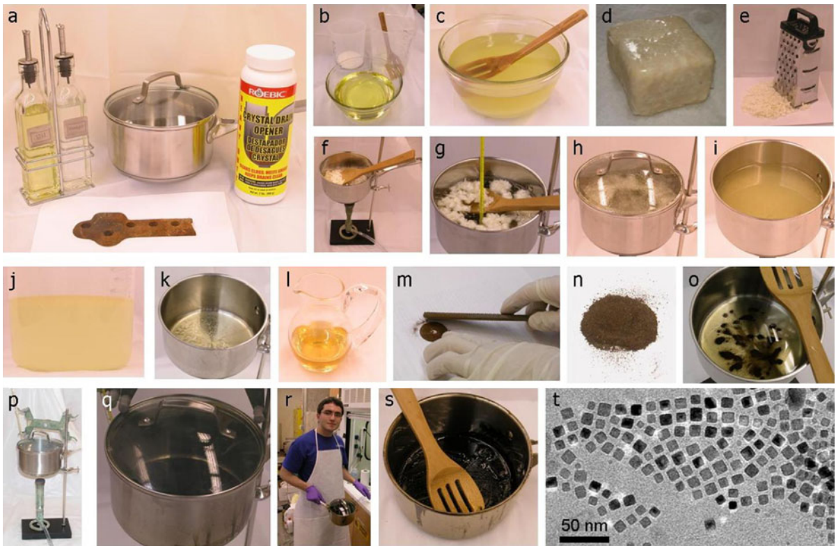
Fig. 6 Scheme of the kitchen synthesis. a Ingredients for a typical nanocrystal synthesis include: oil, vinegar, pan, crystal drain opener, and rust. b, c Synthesis begins with soapmaking, the first step of which is mixing the oil with the crystal drain opener and water. d After curing for 1 day, the soap solidifies. e–h For efficient dissolution in subsequent steps, the soap is ground to a fine powder ( e ), then mixed with vinegar ( f ) while heating on a stove ( g, h ). i, j Once all of the soap is dissolved, the solution forms two layers: a yellow top layer and a cloudy white/yellow bottom layer. k The top layer is the fatty acid
